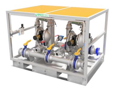
The high-pressure pump was developed for applications requiring fluid pressures in excess of the 100 psi developed by traditional pumps. Compared to a standard diaphragm pump, the 2:1 ratio high-pressure pump can produce up to 200 psi, at about half the flow rate.
