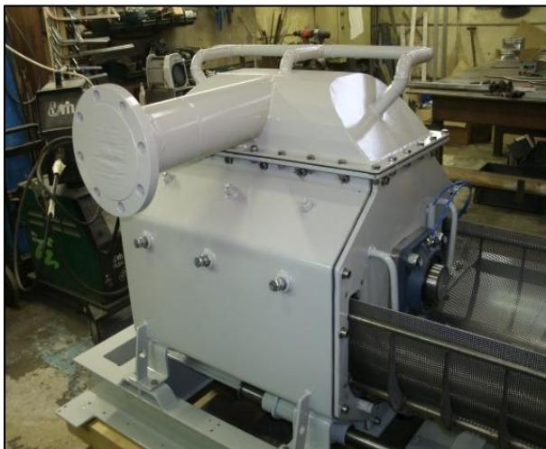
Our MUD Mill HTS-700 is made of steel and intenedt for the specific purpose of crushing drilling cuttings
